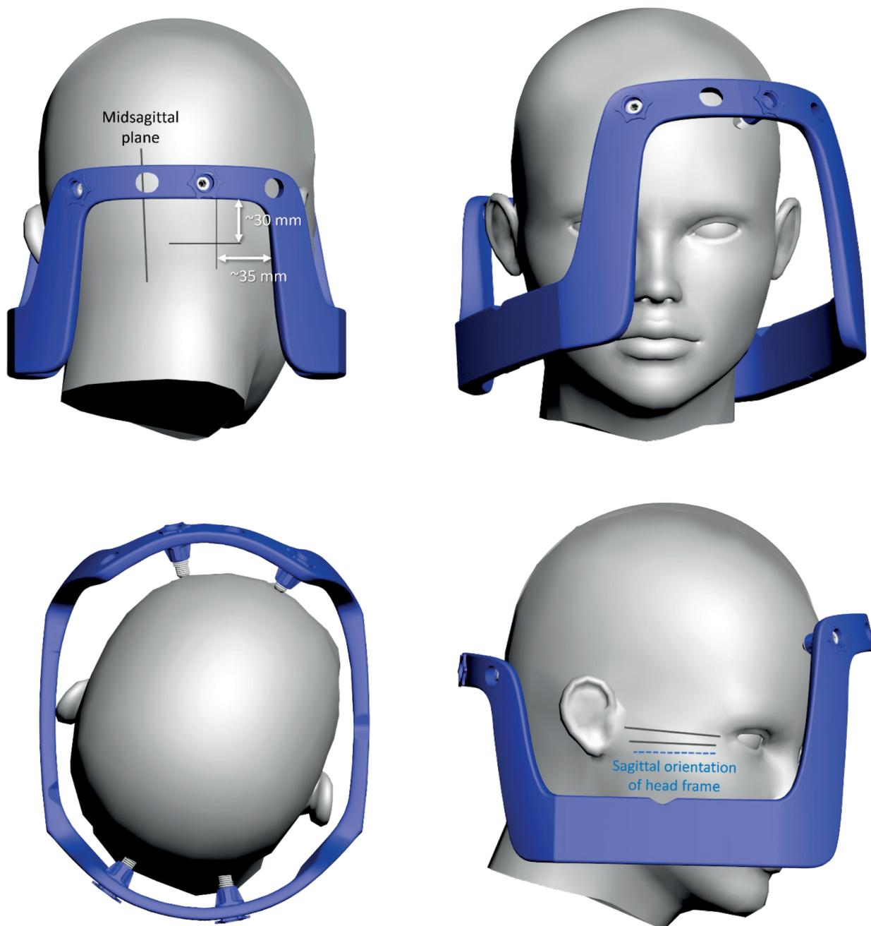
Figure 9. Illustration of head frame positioned according to markings. The frame is mounted with ~25 degrees horizontal rotation and with a few degrees larger sagittal angle than the planned trajectory. The trajectory is located within the posterior window and will be accessible for the stereotactic procedure. Upper left: Posterior view, upper right: frontal view, lower left: superior view, and lower right: lateral view.
