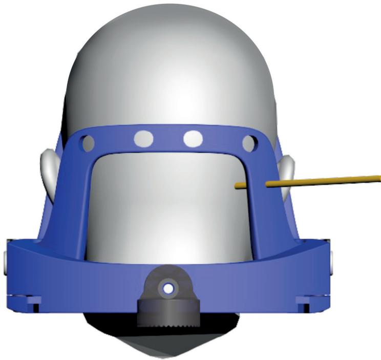
Figure 4. Posterior view of a regularly mounted head frame and frame holder together with a trajectory illustrated with a yellow cylinder. In this case the trajectory is blocked by the right 'post' of the head frame.
