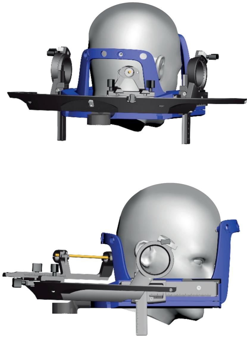
Figure 10. Vantage arc in lateral right orientation. Left) posterior view, and Right) lateral view.
