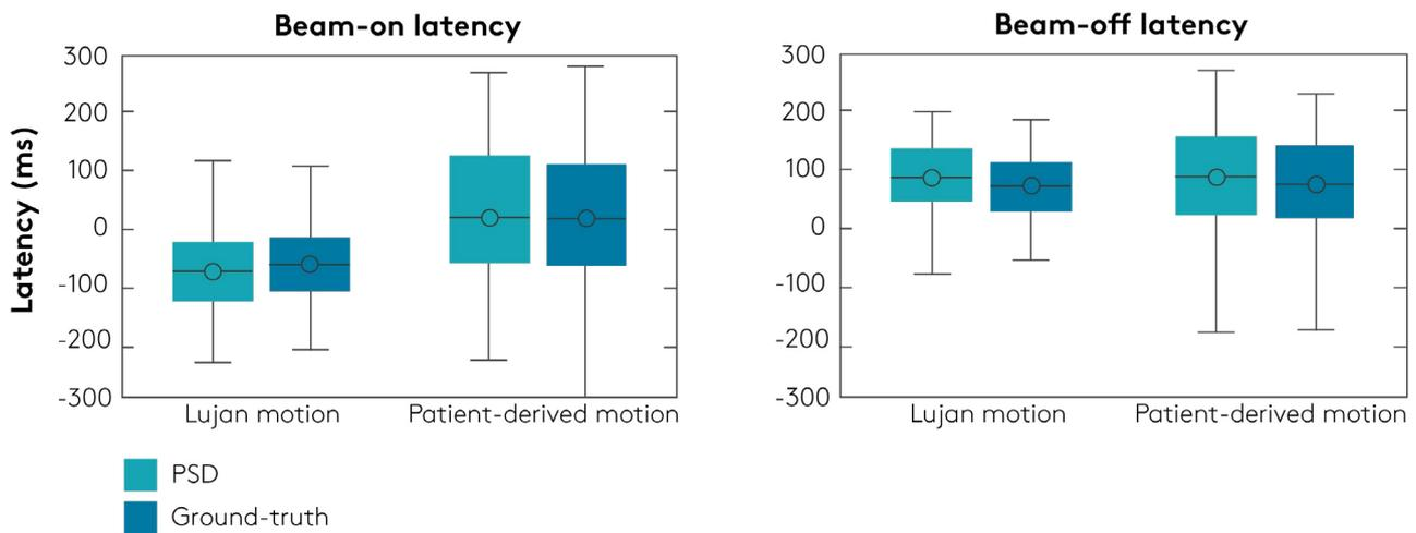
**Figure 7** Beam gating latency based on the MRI 4D scintillator cassette’s PSDs and based on the beam pulses.
